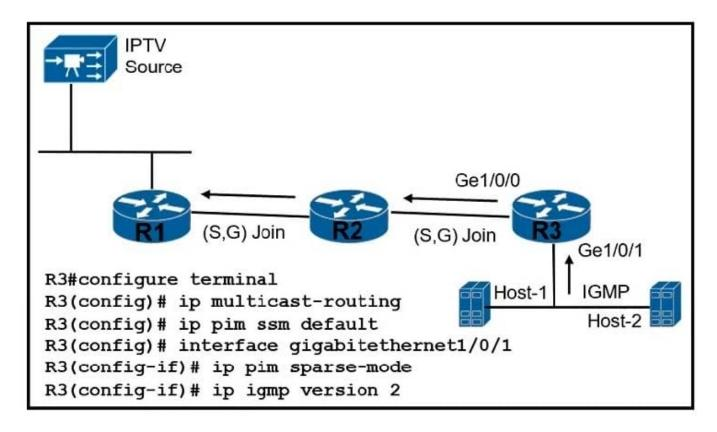
A customer reports that Host-1 is failing to receive streaming traffic from the IPTV source. The engineer has confirmed that hosts on router R2 are receiving traffic normally and that Host-1 is correctly sending subscription messages to join the IPTV stream. Which action must the engineer take to correct the problem?
