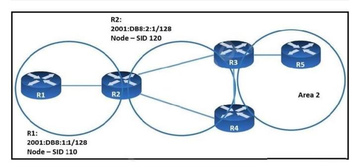
When implementing SRv6, which SID does R2 propagate into area 0 for the prefix 2001:DB8:1:1/128?
