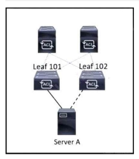
Server A is connected to the Cisco ACI fabric using two teamed interfaces. One interface in a team is configured as active and the other remains in standby mode. When a failover occurs and the standby interface becomes active, it uses its built-in MAC address to send traffic. Which bridge domain configuration must be applied to resolve the issue?
