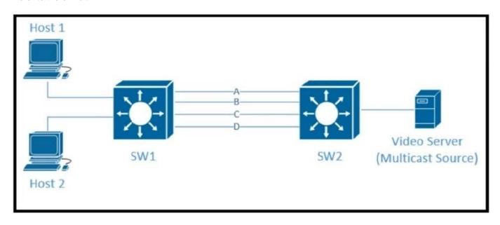
Traffic was equally balanced between Layer 3 links on core switches SW1 and SW2 before an introduction of the new video server in the network. This video server uses multicast to send video streams to hosts and now one of the links between core switches is over utilized.
