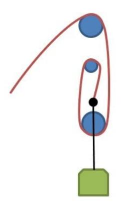
What is the mechanical advantage of this pulley system?
