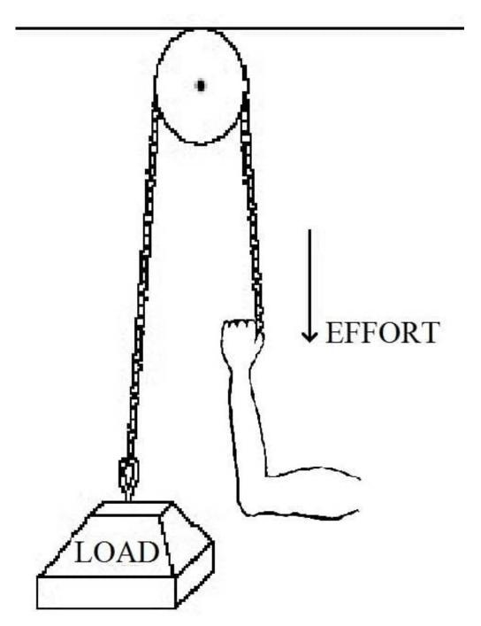
What mechanical advantage does the block and tackle arrangement in the above figure give?
