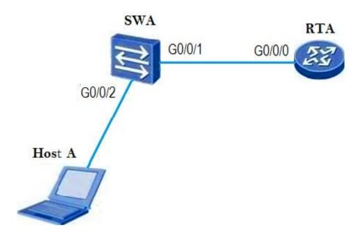
A host has established a telnet connection with the router attached to interface G0/0/0. Which of the following statements are correct? (Choose two)
