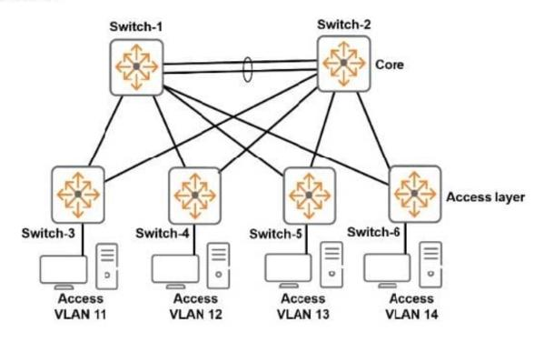
This exhibit shows the topology for a company campus LAN. Each access layer switch will be the default router for the devices connected to it. The company needs to permit the following:
