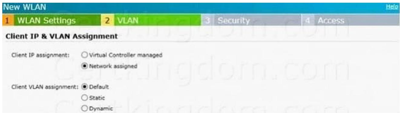
The exhibit shows settings for a WLAN on an Aruba Instant cluster. To which VLAN is wireless user traffic assigned?
