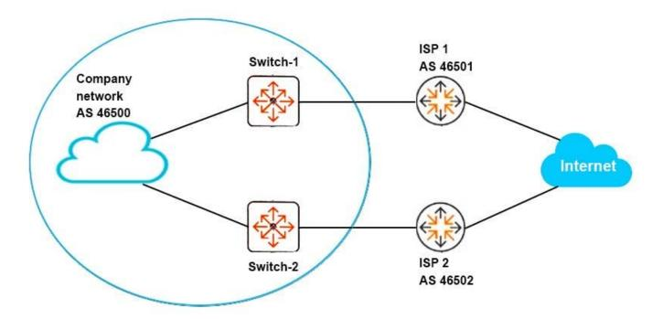
Switch-1 and Switch-2 are AOS-Switches, which are iBGP peers. ISP 1 and ISP 2 advertise some routes to the same Internet destinations. Switch-1 and Switch-2 must select between these routes based on AS path length.
