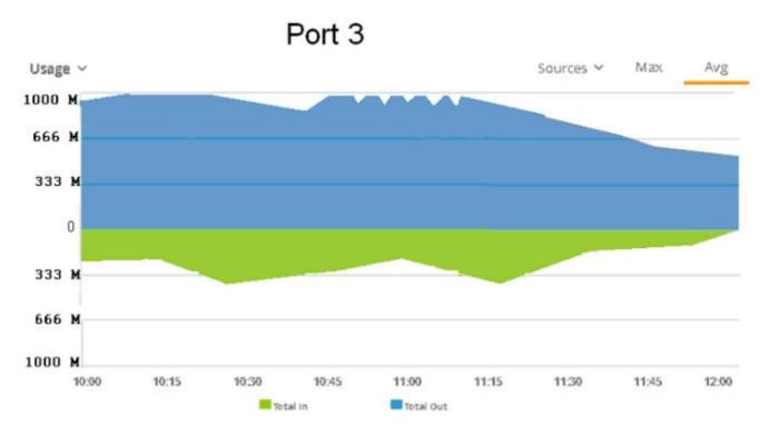
A customer needs a wired network upgrade and has complained about performanceissues. The architect collectedinformation about traffic now on several switch ports in different locations across the network, and the results are shown in the exhibit. Each of these ports is a 1Gbps port.
