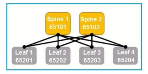
For a fully configured and functional IP fabric underlay as shown in the exhibit, how many external BGP
