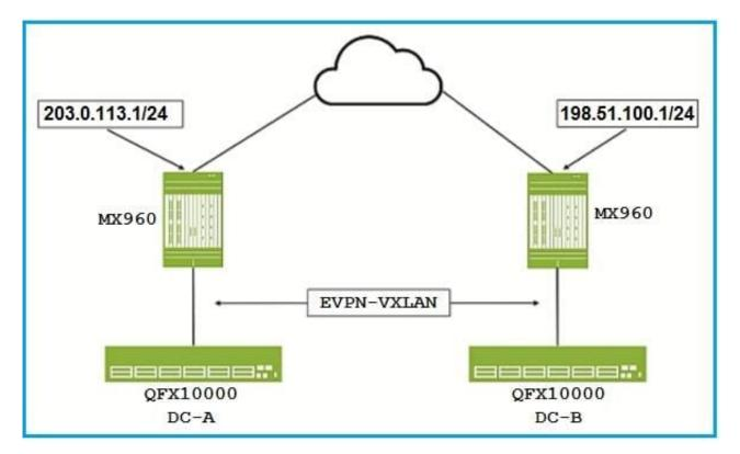
You are designing a Data Center Interconnect to transport VXLAN traffic between DC-A and DC-B.
