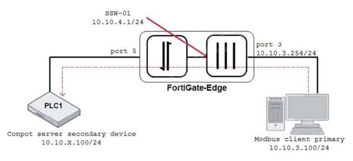
An OT architect has implemented a Modbus TCP with a simulation server Conpot to identify and control the Modus traffic in the OT network. The FortiGate-Edge device is configured with a software switch interface ssw-01.
