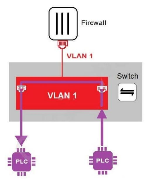
In the topology shown in the exhibit, both PLCs can communicate directly with each other, without going through the firewall.
