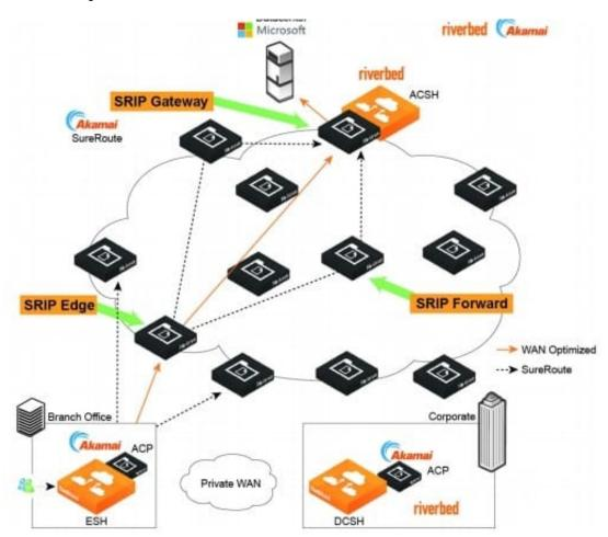
Although the DCSH encapsulates the traffic, it plays no role in the SSL optimization process. SSL optimization still takes place between the ESH appliance and the ACSH. Ensure that you establish the SSL peering trust between them.
