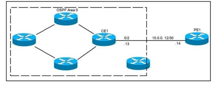
CE1 is the gateway router into the provider network via PE1. A network operator must inject a default route into OSPF area 0. All devices inside area 0 must be able to reach PE1. Which configuration achieves this goal?
