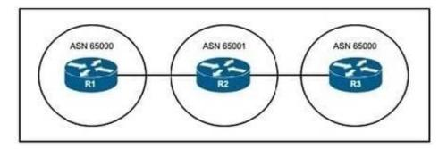
An engineer is troubleshooting an issue with this network and notices that prefixes from R3 are missing on the R1 routing table Due to repeated ASN when the 10 0 0 0\\'8 prefix from R3 arrives at R1, BGP automatically rejects it There is no prefix-list on R1 which blocks the traffic from R3 What should the engineer do to fix the problem so that BGP allows that prefix on R1?
