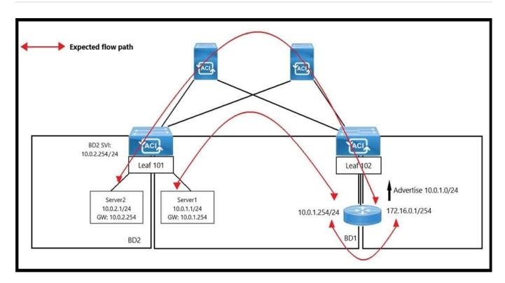
An engineer wants to initiate an ICMP ping from Server1 to Server2. The requirement is for the BD1 to enforce ICMP replies that follow the expected path. The packets must be prevented from taking the direct path from Leaf1 to Server1. Which action must be taken on BD1 to meet these requirements?
