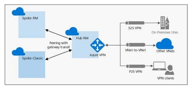
The following diagram shows how gateway transit works with virtual network peering.
