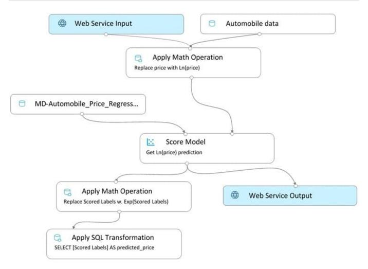
You need to modify the inference pipeline to ensure that the web service returns the exponential of the scored label as the predicted automobile price and that client applications are not required to include a price value in the input values.
