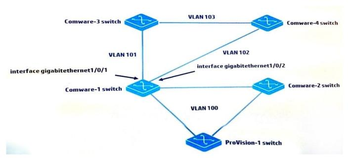
MSTP is configured on all switches shown in the exhibit. The Comware-1, Comware-3, and Comware-4 switches are set up for OSPF. Comware-1 and Comware-4 switches fail to achieve neighbor adjacency. The network administrator analyzes the issue and determines that MSTP is blocking on port gigabitethernet1/0/2 on Comware-1.
