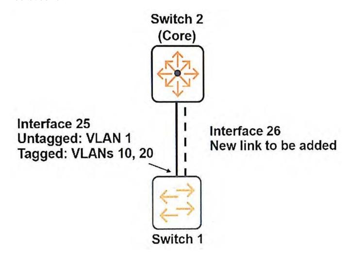
Switch 1 shown in the exhibit is an ArubaOS switch that has an uplink to the network core on interface 25.
