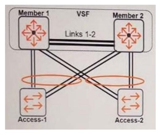
Which feature should the network administrator configure on the Virtual Switching Framework (VSF) fabric to prevent issues if Links 1 and 2 fail?
