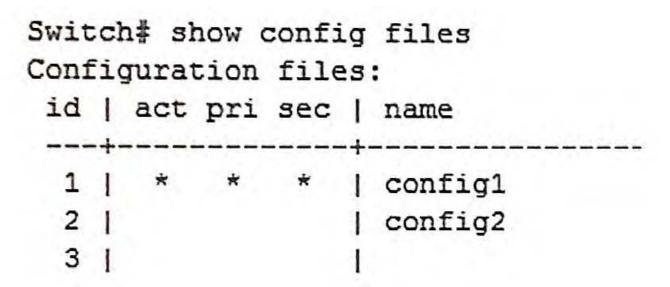
A network administrator views the configuration files on an ArubaOS switch and sees the output in the exhibit. The administrator enters this command: Switch# boot system flash primary config config2
