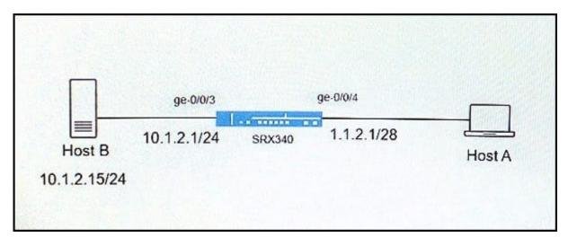
Host A is attempting to connect to Host B using the domain name, which is tied to a public IP address. All attempts to connect to Host B have failed. You have examined the configuration on your SRX340 and determined that a NAT policy
